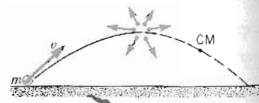
FIGURE 6-4 A grenade explodes while in a trajectory of projectile motion. Because there has been no external force involved in the explosion, the motion of the center of mass is unchanged.
