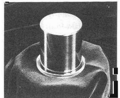
The standard kilogram, a platinum-iridium cylinder kept at the International Bureau of Weights and Measures in Sèvres, France.
