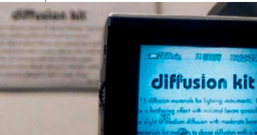
FIGURE 3: To ensure correct focus, it is useful to zoom in on sample text placed at the distance of the screen.
