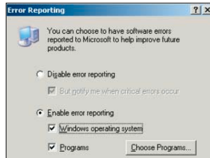
FIGURE 2: You can configure WER not to send reports or to send reports only for certain programs or types of programs.
