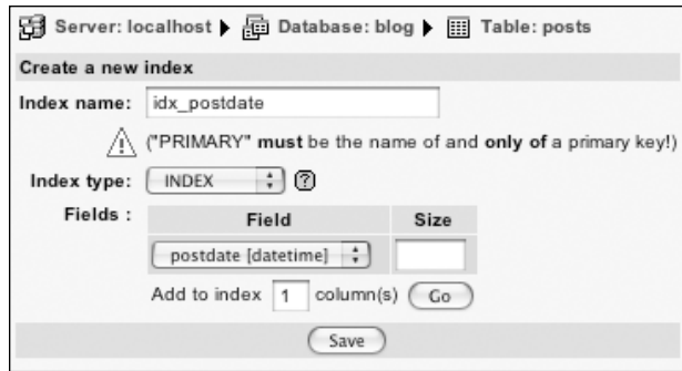
Figure 7-23. Adding an index to the postdate field in phpMyAdmin
