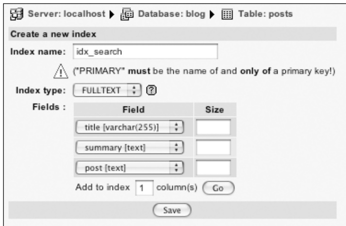
Figure 7-21. Adding a fulltext index to the posts table in phpMyAdmin
