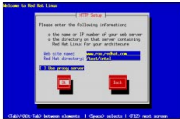
Figure 5.8: Installing via HTTP
