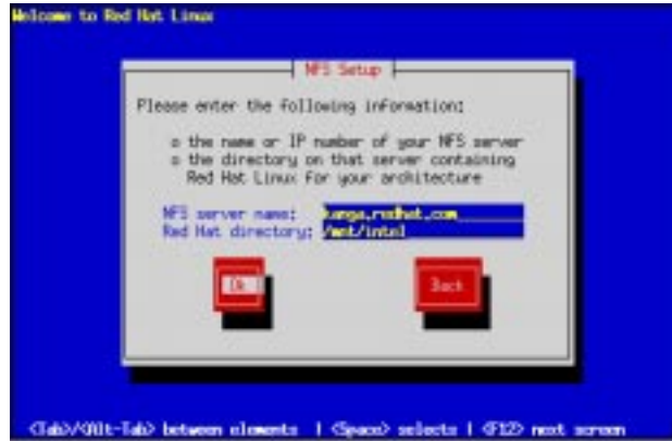
Figure 5.6: Installing via NFS
