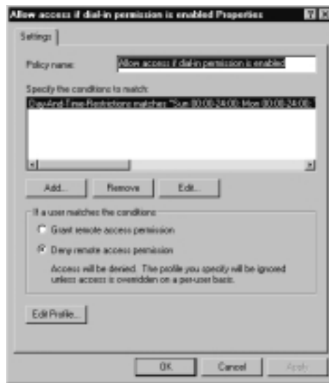
Figure 9.2 Grant or Deny Remote Access Permission Options within the Remote Access Policies
