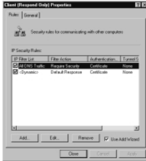
Figure 8.9 Client (Respond Only) Properties with a Custom Rule Added for DNS Traffic
