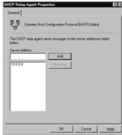
Figure 9.7 Configuring DHCP Relay on RRAS so Remote Access Clients Receive DHCP TCP/IP Options
