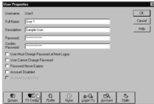
Figure 5.7 Using User Manager for Domains to Configure NT4 Accounts for Windows 2000 Terminal Services
