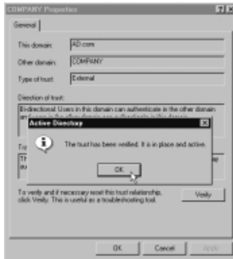
Figure 1.9 Verifying an Active Directory Trust Current Status
