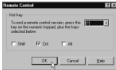
Figure 5.12 Configuring or Accepting the Remote Control Hot Key to End a Remote Control Session
