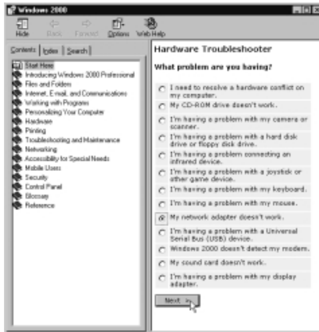
Figure 2.22 Hardware Troubleshooter Being Used to Help Diagnose and Remedy Problems with the Network Adapter
