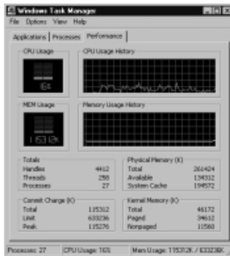
Figure 3.27 Using Windows Task Manager Performance View
