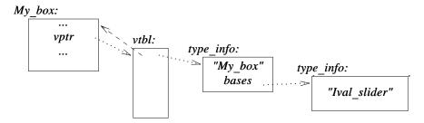
The dashed arrow represents an offset that allows the start of the complete object to be found given only a pointer to a polymorphic sub-object. It is clear that *dynamic\_cast* can be efficiently implemented. All that is involved are a few comparisons of *type\_info* objects representing base classes; no expensive lookups or string comparisons are needed.
