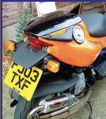
Butchy's Dragster in Telford. Pictured here with a seat pod and chopped down number plate bracket
