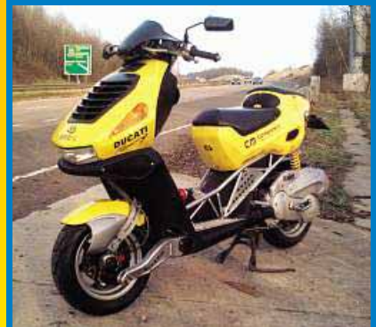
From Croydon, here's Mark Tatum's Ducati Breil-styled Dragster fitted with all the usual Malossi go-faster goodies plus a Scorpion pipe and Bitubo front shock absorber
