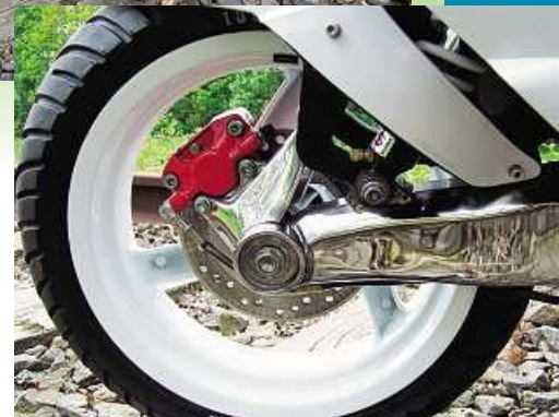
A Pug Speedfight shock absorber has been fitted to the polished front swing-arm.
