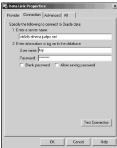
Figure 26-5: Specifying values for the key connection properties.
