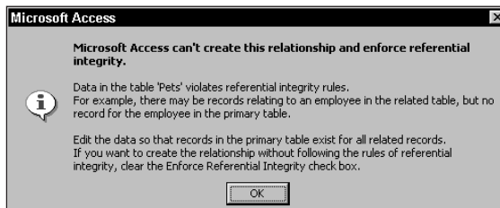
Figure 6-7: A dialog box warning that referential integrity cannot be created between two tables due to violations in some of the records between the two tables — one or more Pets without a Customer is probably the problem
