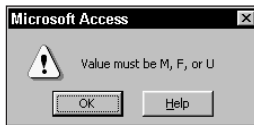
Figure 7-8: The data validation message for the Pets Gender field appears anytime the user fails to enter an M, F, or U in the field.
