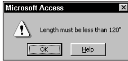
Figure 5-16: A data-validation warning box. This appears when the user enters a value in the field that does not match the rule specified in the design of the table.
