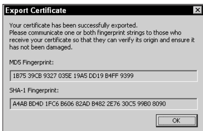
Figure 14-4: The Export Certificate contains fingerprints intended to be shared with your community certificate holders. This information does not compromise your private certificate.
