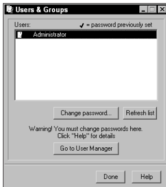
Figure 5-28: The Users and Groups dialog box enables me to establish file-sharing privileges.
