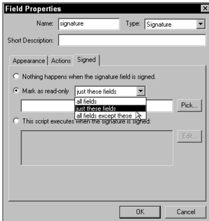
Figure 13-17: The Signed tab offers options for signature fields where a digital signature can be defined for a field and actions associated with applying a signature are established.
