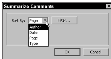
Figure 8-34: The Summarize Comments dialog box enables you to create a separate PDF file with the comments summarized according to a sort order made from a pull-down menu.
