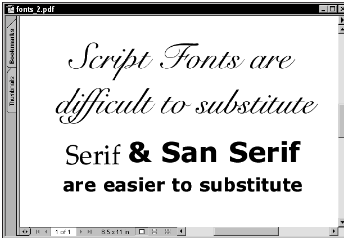
Figure 3-4: If the actual font(s) are installed or embedded in the PDF file, the display and printed file includes the original fonts.
