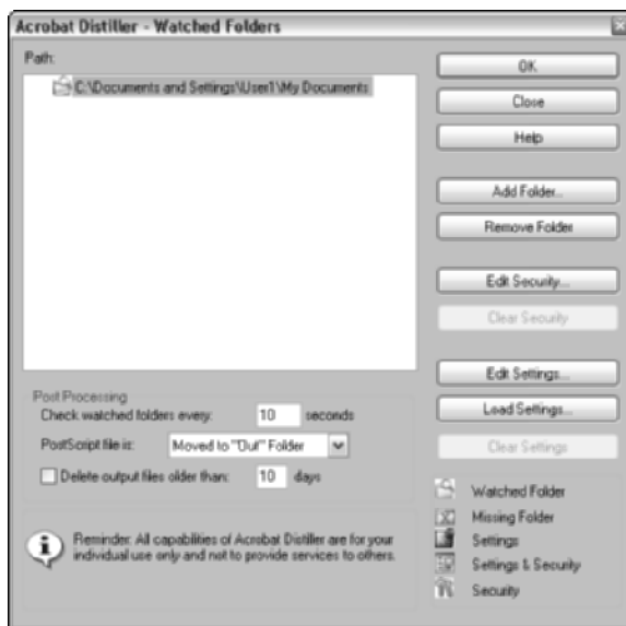
Figure 4-13: Setting up watched folders in the Acrobat Distiller - Watched Folders dialog box.
