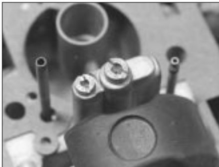
12.13c Secondary main jet (left) and TM fuel jet (right) tightened in the cover
