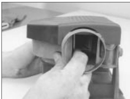
16.1 Check for binding of the flap in the airflow meter as it nears closing position or wide-open position. Any hesitation or binding will cause erratic idle conditions, rich fuel mixture or poor acceleration and throttle response (airflow meter removed for clarity)
