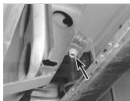
6.10b Remove the retaining strap bolts (one arrowed) and lower the fuel tank
