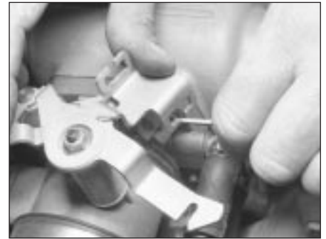
9.10a Rotate the throttle valve and remove the cable end from the slotted portion of the valve
