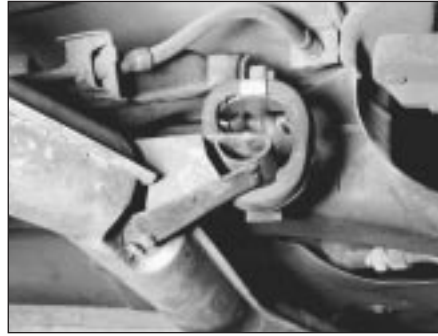
22.1 A typical exhaust system rubber mounting
