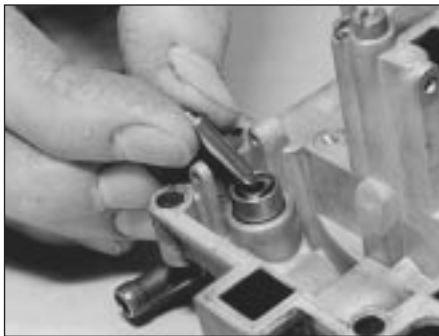
12.12b . . . then lift out the needle valves, keeping all components identified side for side
