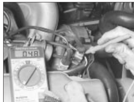
19.4 Check for a voltage signal on the black/yellow wire of the thermotime switch when the ignition is on
