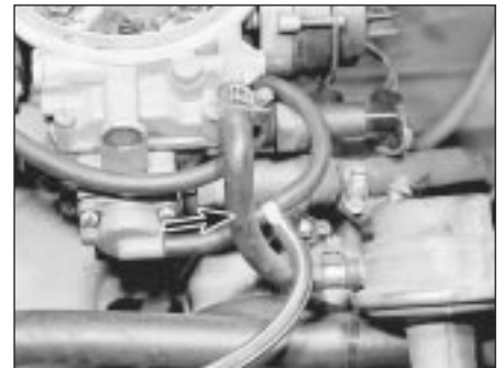
11.8 Disconnect the fuel supply hose (arrowed)
