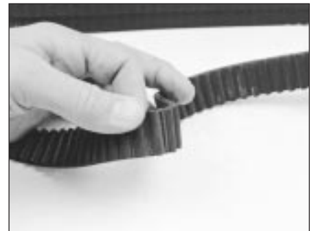
10.13a Inspect the timing belt carefully for cracking, as shown here. . .
