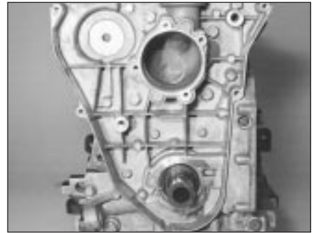
14.14a Front end cover and oil pump in position on the front of the M40 engine
