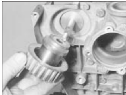
14.8 Removing the timing belt tensioner (M40 engine)
