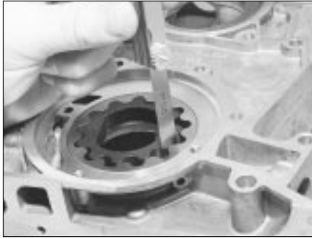
14.24b Measuring the clearance between the oil pump outer and inner rotors (M40 engine)
