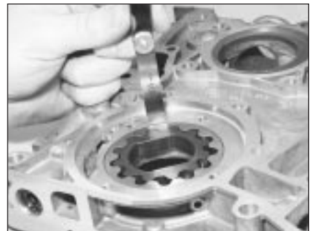
14.24a Measuring the clearance between the oil pump body and the outer rotor (M40 engine)
