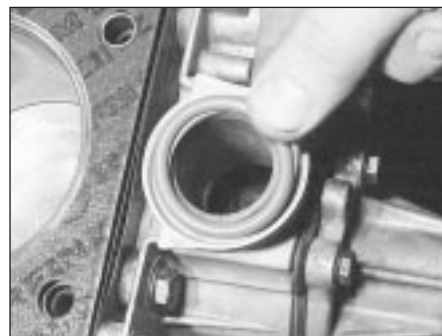
12.26 Fitting a new rubber O-ring in the groove in the top of the oil pump/front end cover on the M40 engine
