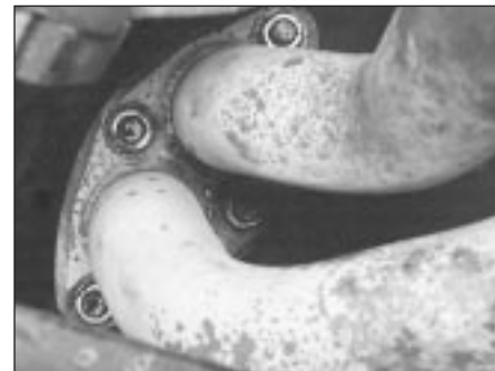
6.5b Exhaust manifold-to-downpipe flange (M40 engine)
