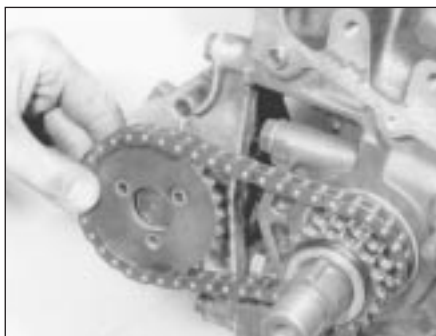
14.2 On M10 and M30 engines, remove the three bolts that hold the driven gear to the oil pump, and remove the gear
