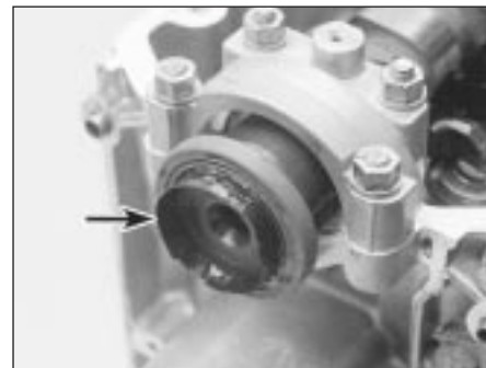
11.14 Fitting a new camshaft oil seal on the M40 engine (note the adhesive tape around the end of the camshaft to protect the seal)
