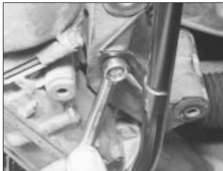
13.7b Removing the oil dipstick tube bracket mounting bolt
