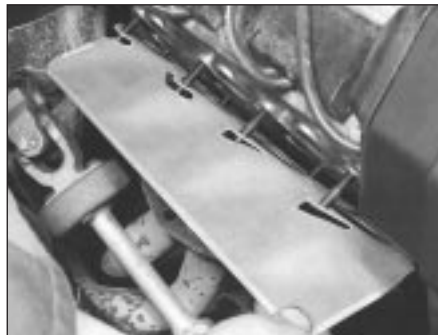
6.7b Removing the exhaust manifold gasket (M40 engine)
