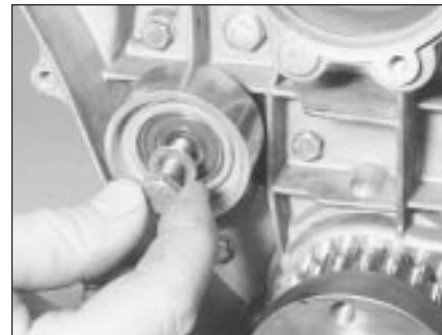
14.11b Removing the guide roller from the front end cover (M40 engine)
