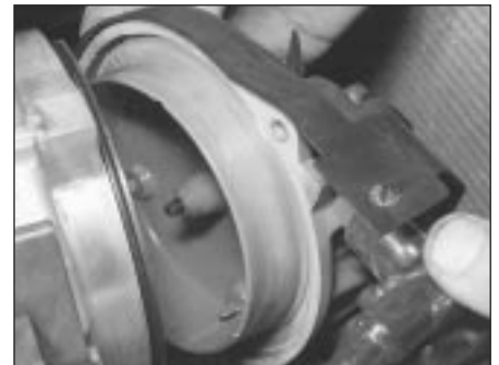
9.6a Unbolt the distributor cap (M40 engine) . . .
