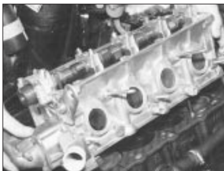
12.28 Lowering the cylinder head onto the block (M40 engine)
