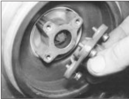
9.6b ... then unbolt the rotor ...
