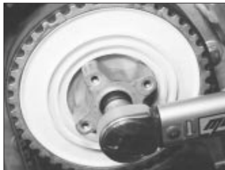
10.27 Tightening the camshaft sprocket retaining bolt on the M40 engine
