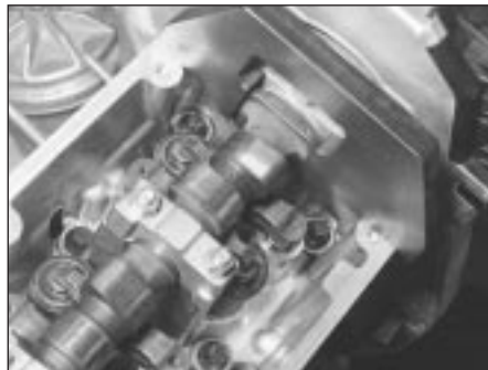
10.11b The BMW camshaft-holding tool in position on the M40 engine
