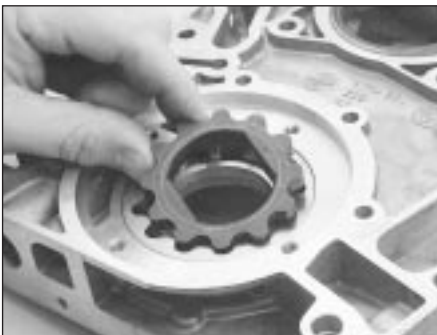
14.22a Removing the inner rotor . . .
