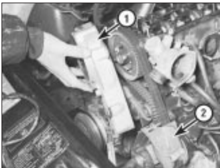
9.9a Remove the upper timing belt cover first, then the lower cover (M20 engine)
