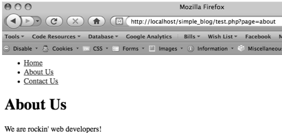
Figure 3-2. The About Us page is loaded when the page=about query string is passed in the URL
